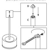
**4** Make a hole in the floor, recommended Ø35mm diameter. Minimum depth of 200mm depending on the type of soil.
