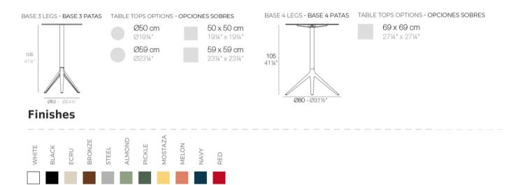
Powder coated aluminum base with non collapsable attachment made of polyamide and fiber glass
